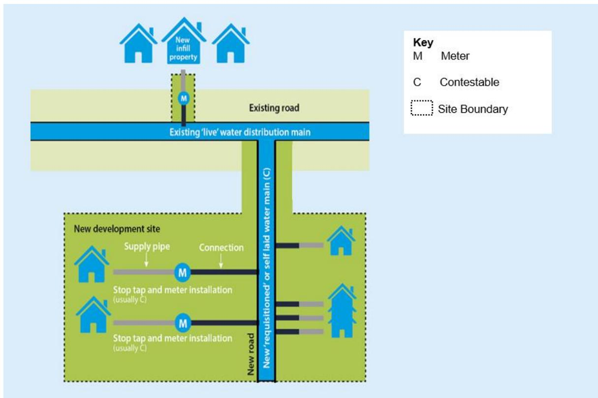
The pipework we lay (the comm. pipe) will run from the location of the meter to our existing main which is normally situated in the adjacent highway (for infill properties) or through the development site if the main has been recently laid. The customer is responsible for laying the pipework from the property up to the boundary shown as the supply pipe on the diagram above.
