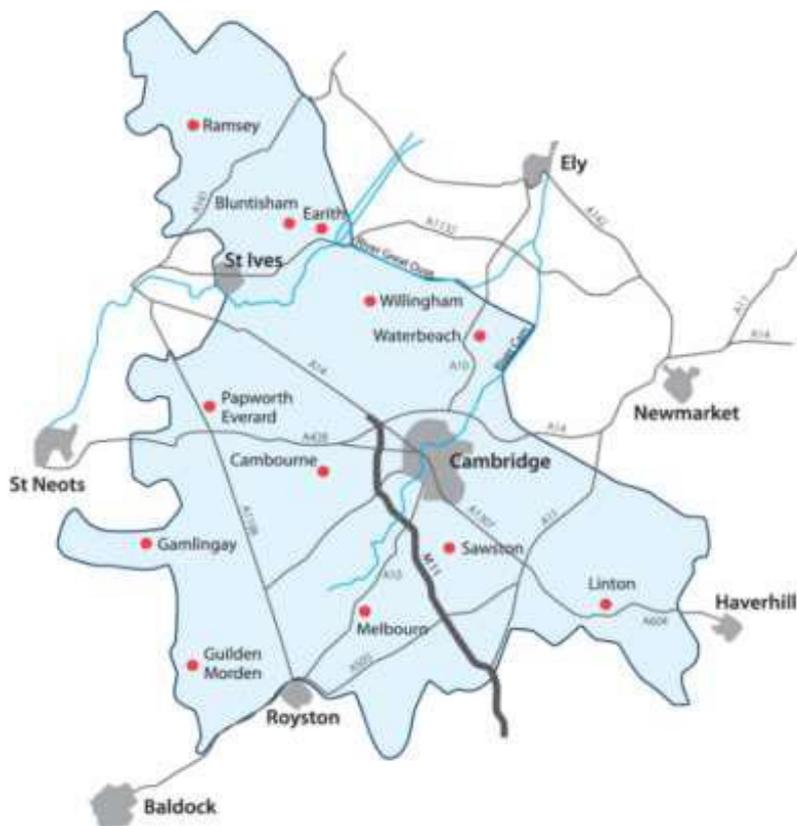
The network comprises five supply zones – the Cambridge zone is the largest of these, in terms of both supply and demand. Sources which supply water direct into this zone provide more water than is needed there to meet demand, so the surplus water is transferred to other zones as required.
