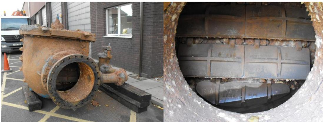
Figure 8: 36" multi-gate non-return valve removed during 2011
