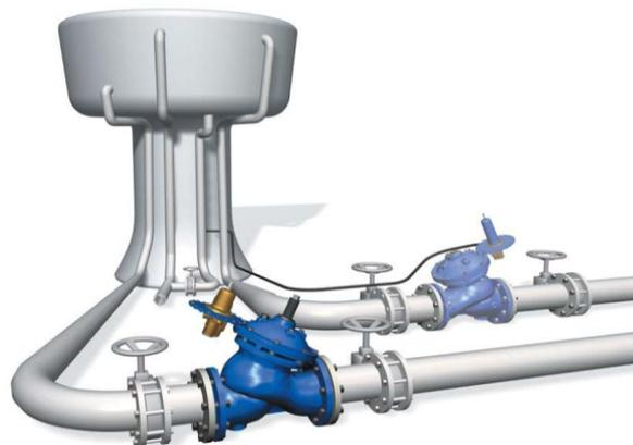
Figure 9: example setup of auto valves
