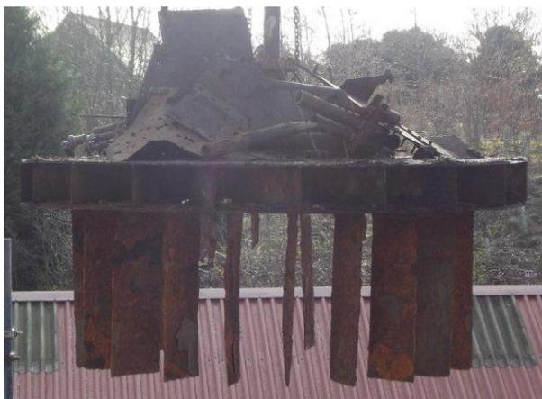
Each clarifier structure has a central stirrer which is suspended from its drive motor above by a single drive shaft.
